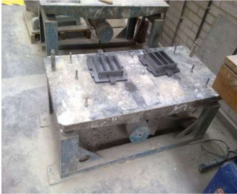
Figure 6:Electrical vibrating machine
